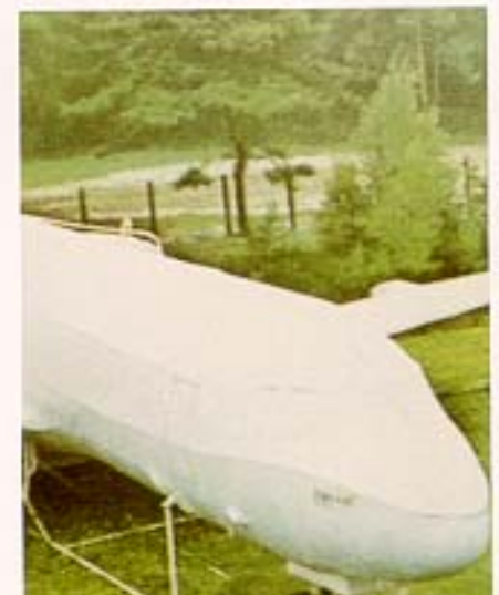
Fokker B.V. Aircraft are cocooned and dehumidified to prevent corrosion during storage.
