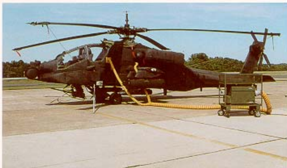
U.S. Army, Dehumidification of AH-64 Apache for protection of electronic systems.
