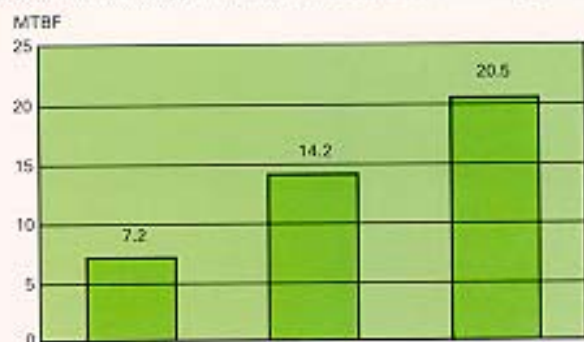
Fig 2 Aircraft J-35 Draken. Evolution of faults. Comparison MTBF, radar and cabin equipment.
